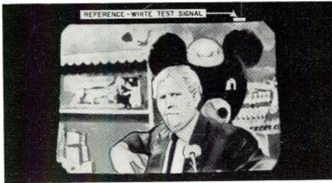
Fig. 7. Photo of an actual CBS program, showing the position in the raster of the reference-white signal, upper right.
