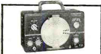
Model G-30 RF SIGNAL GENERATOR KIT • 160 Kc to 240 Mc in 8 bands • 120 Mc fundamental output Net Price: $28.50 Model G-30-PC: Same as Model G-30 but with pre-calibrated front end. Net Price: $35.50
