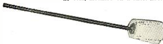
Fig. 2. Tube tapper made from #8 bottle cork, mounted on a short fiber rod.
